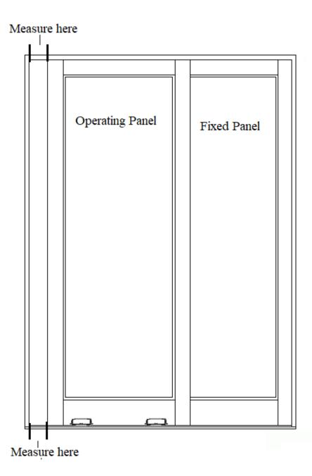
Open door panel 1 to 2 inches Measure the distance from the Jamb to the panel on both top and bottom.
